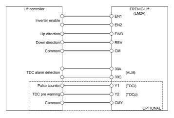
Figure 7. Wiring example for TDC function
