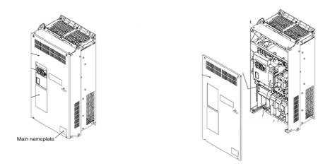
Figure 3. Name plate position in capacities from 0060 to 0091.
