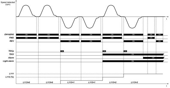
Figure 6. Basic function time chart of TDC function
