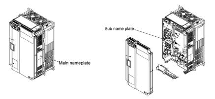
Figure 2. Name plate position in capacities from 0039 to 0045.
