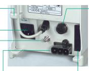
Multi-Function-Connector (MFC) Connection for staff call, ambulances (12 V DC) and interface for fm anaesthesia/fm intensive.
