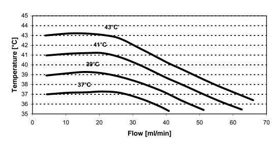
AP 260S, Settings 43/41/39/37 °C, appliance outlet temperature, initial temperature 20°C
