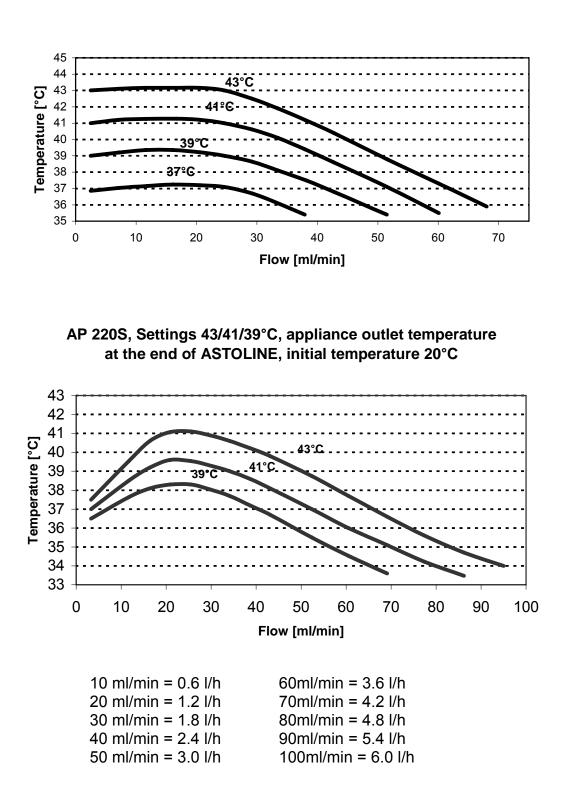
AP 220S, Settings 43/41/39/37°C, appliance outlet temperature, initial temperature 10°C
