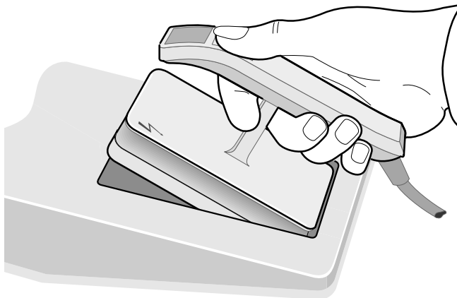
Figure 4-8. Returning the paddles to their compartments
