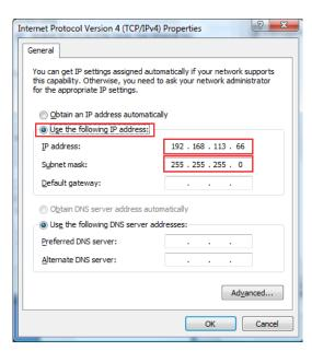
• Input the default Cadwell® IP address used for all our machines. It is **192.168.113.66**. The default Subnet Mask can be used of **255.255.255.0**.
