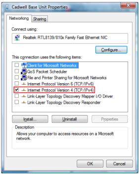
• Then double-click on that protocol and change the radial button from "Obtain and IP address automatically" to "Use the following address."
