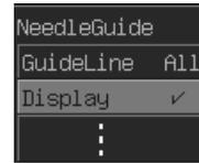
Roll the trackball to highlight the [Display] item. Press the 『Set』 or the 『Back』 key to toggle between On and Off.
